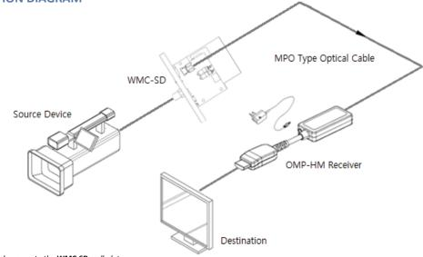
$\textbf{\textit{NOTE:}} \ \textit{The installer must supply power to the WMC-SD} \ \textit{wall plate}$
